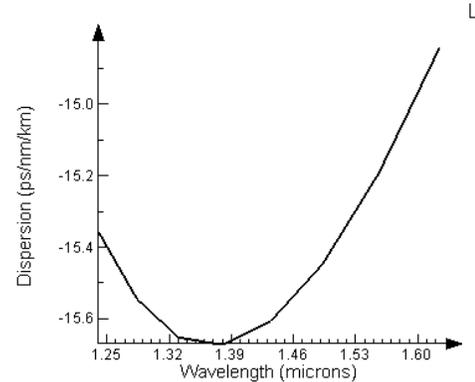
**Fig.6(b):** Dispersion for the new design
