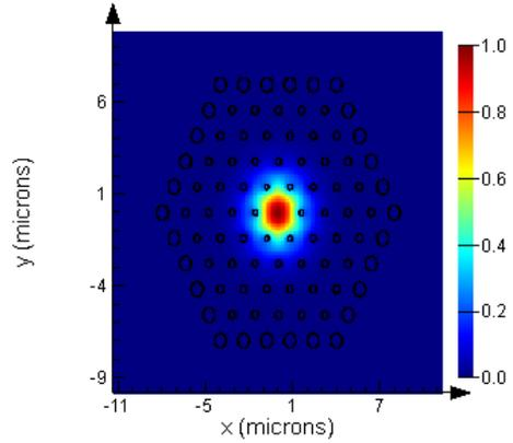
**Fig. 5** Electric Field Intensity through the fundamental mode.
