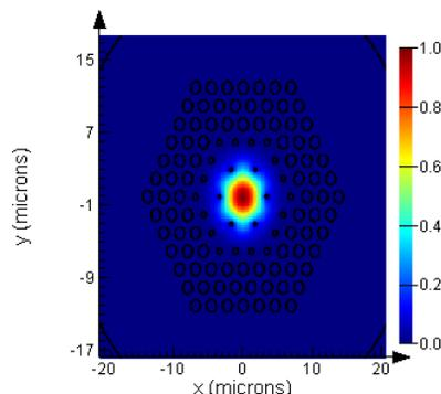
Fig.3 Electric field intensity in fundamental mode
