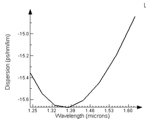
**Fig.6(b):** Dispersion for the new design
