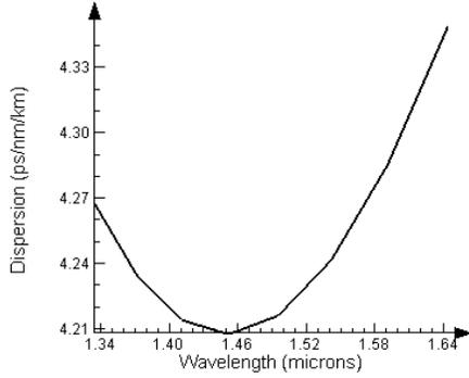
**Fig.4(c):** Dispersion-Wavelength graph
