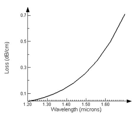
**Fig. 6(a):** Confinement loss for the new design
