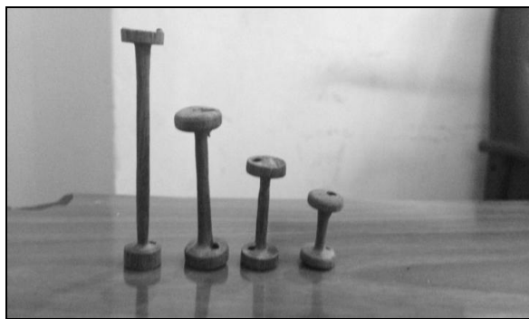
Fig. 1 Wooden spacers used during the blasting experiments
