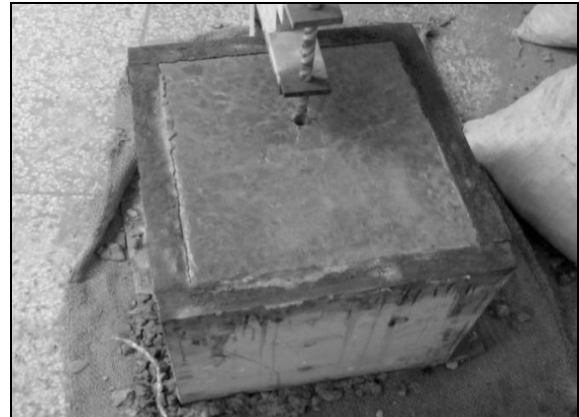
Fig. 2 Concrete block inside the wooden mould with a built-in hole assembly
