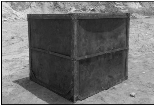
Fig. 4 Metallic blasting chamber with reinforced rubber walls
