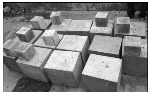
Fig. 3 Smaller concrete blocks along with model blocks for UCS testing.
