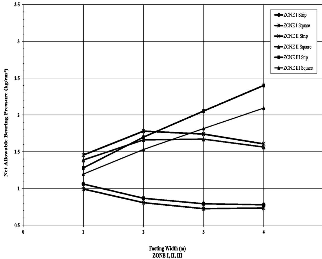
Fig.7: Foundation Proportioning Curves for Zone-I, II and III
