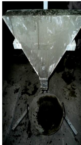
Fig. 13 V Funnel Test
