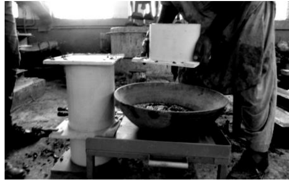
Fig. 11 Column Segregation Test
