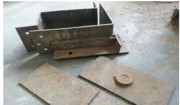
Fig. 6 Mold for casting bricks
