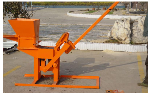
Fig. 7 Manual compression machine for bricks
