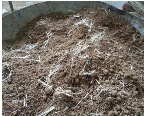
Fig. 5 Mixing of jute with soil
