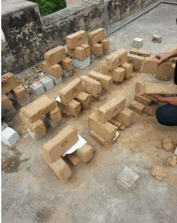
a) Stacking of bricks in Open Air
