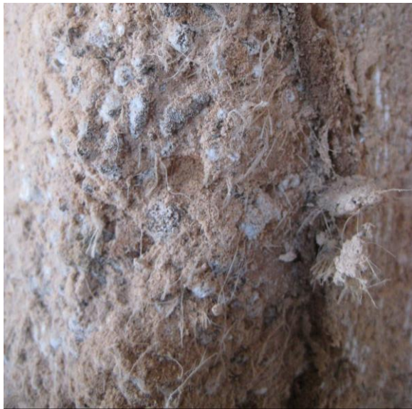
Fig. 1 Jute fibers used in mortar
