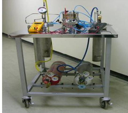
Figure 1: Fuel cell test system.
