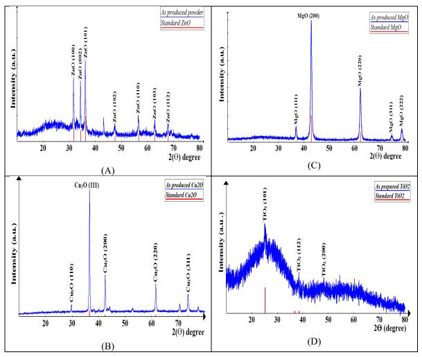
Fig.1: XRD patterns the powders of: A. ZnO, B.Cu<sub>2</sub>O, C. MgO and D. TiO<sub>2</sub>
