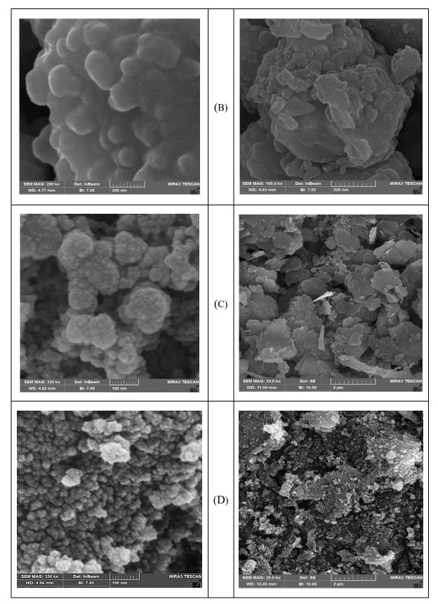
Fig. 2: SEM images of prepared nanoparticles for (A). ZnO, (B) Cu<sub>2</sub>O, (C) MgO and (D) TiO<sub>2</sub>
