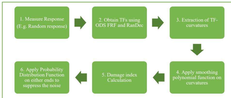
Fig. 5: Proposed methodology for response-only damage detection
