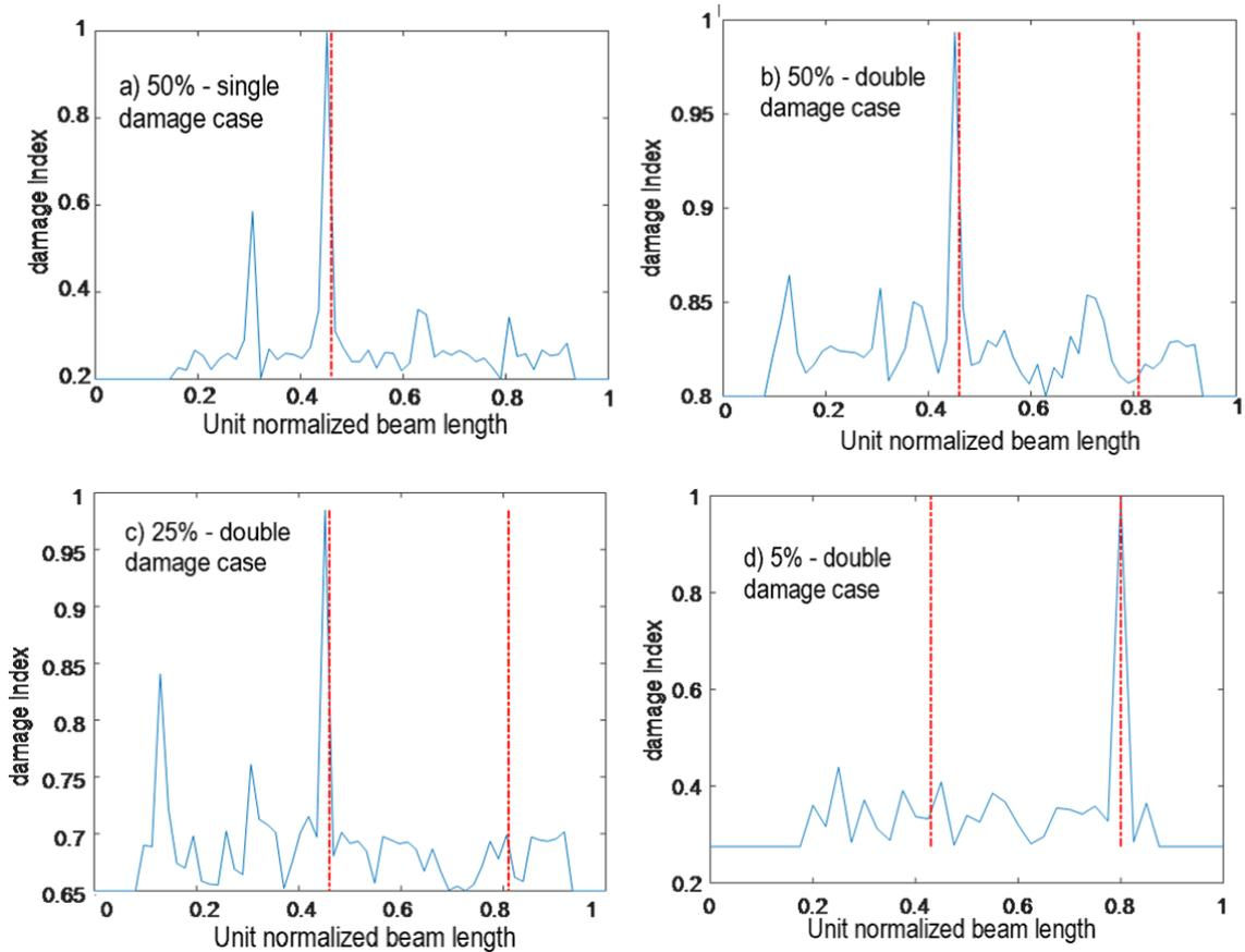
Fig. 13: Damage indices obtained from FRFs
