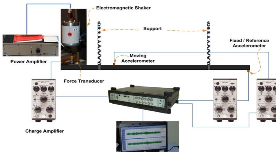
Fig. 6: Schematic diagram of the experimental setup
