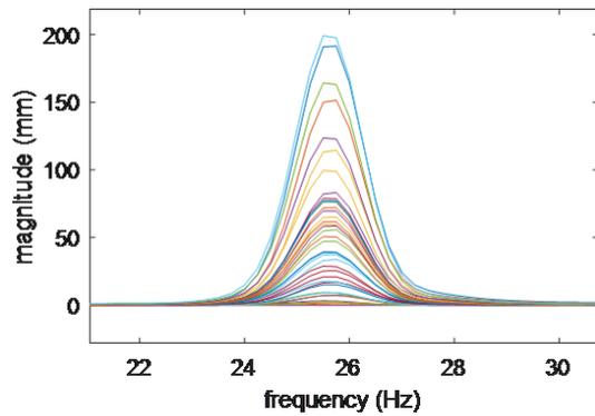
**Fig. 4:** Frequency range of 1st Resonance
