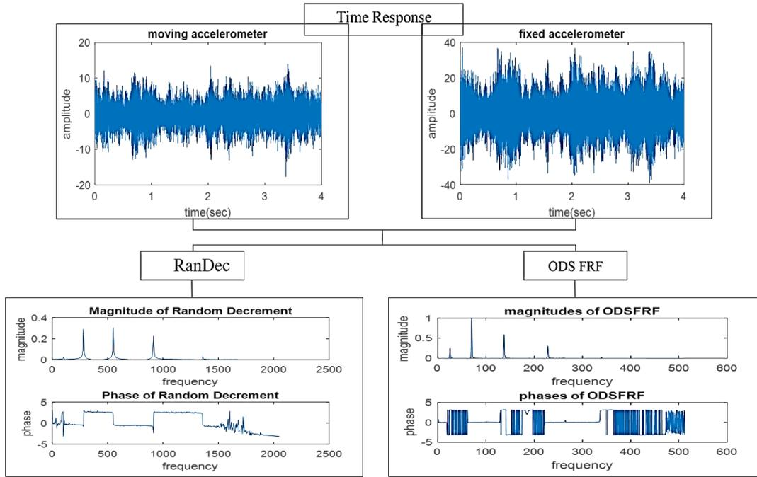
Fig. 7: FRFs comparison of ODS FRF and RanDec at Point 3
