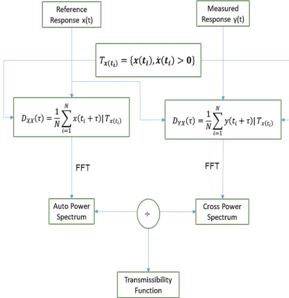
**Fig. 2:** Schematic Flow chart of Random Decrement Technique
