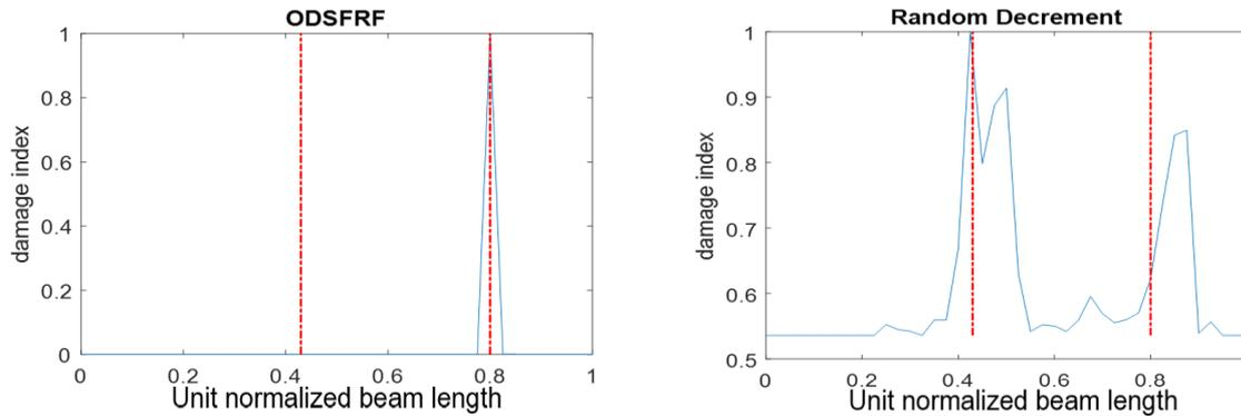
**Fig. 11:** Damage Case IV—5% thickness reduction (double damage)
