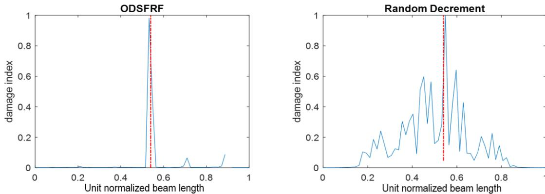
Fig. 8: Damage Case I—50% thickness reduction (single damage)
