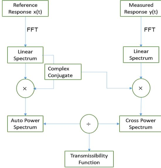
**Fig. 1:** Schematic Flow Chart for ODS FRF
