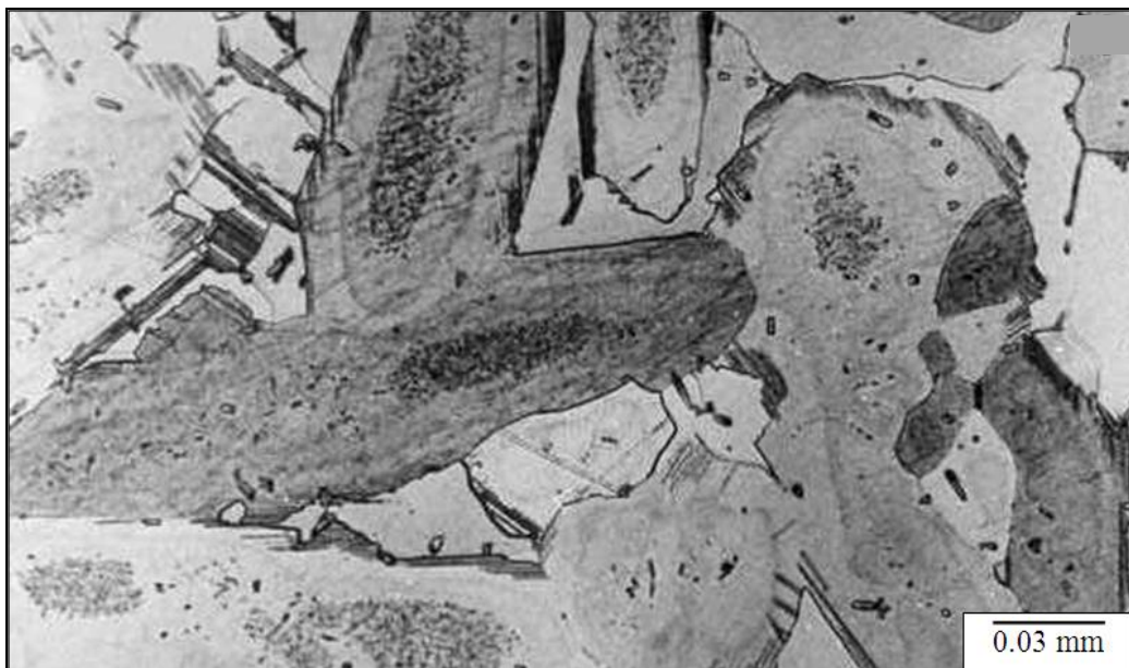
Figure 9: Microstructure of the sample quenched from 550°C, showing a microstructure similar to the as-cast alloy.
