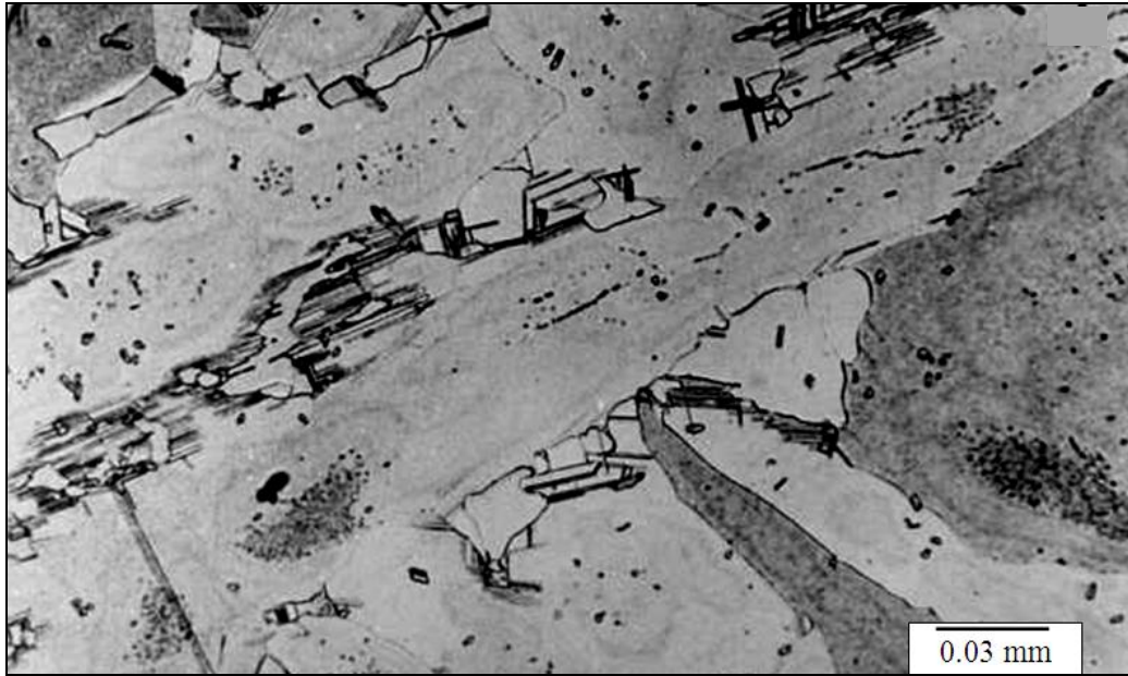
Figure 8: Microstructure of the sample quenched from 650°C, showing the \alpha , \gamma_2 and twin-like structure along \alpha / \gamma_2 grain boundaries.
