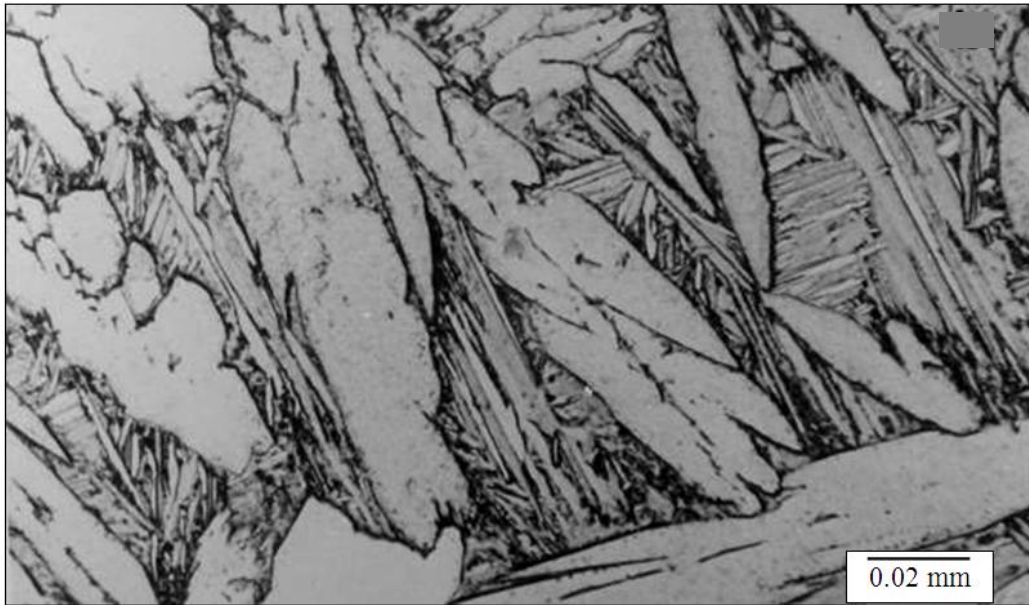
Figure 5: Microstructure showing the Widmanstätten growth of \alpha -phase in the \beta matrix.
