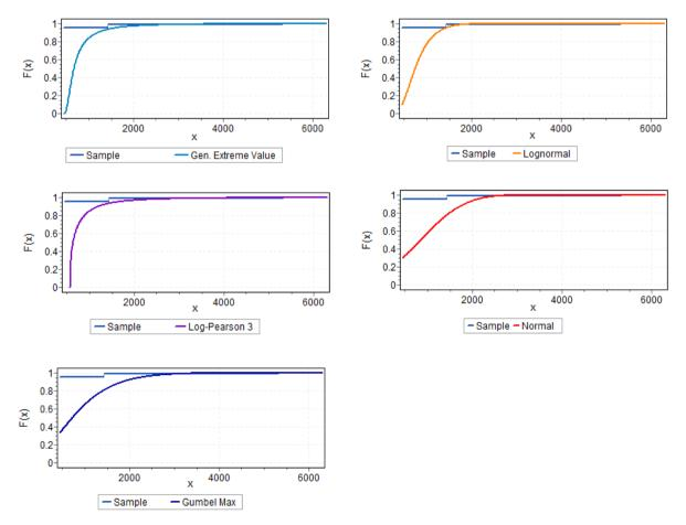
Fig. 4: Cumulative Distribution Function Plot of Different Statistical Distributions
