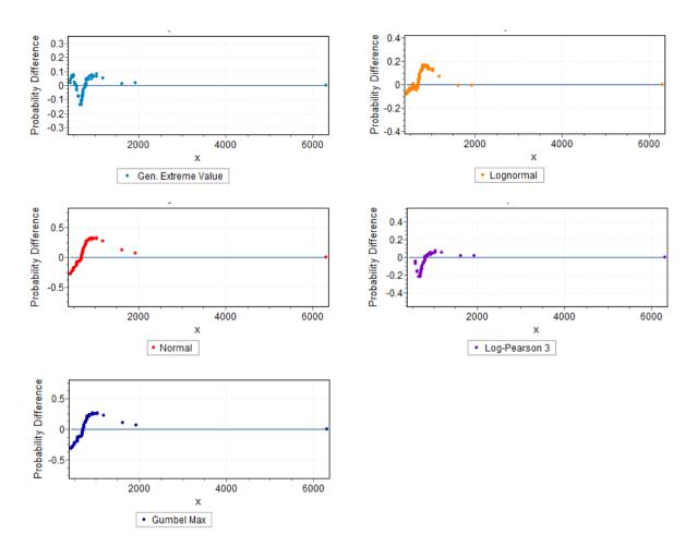
Fig. 7: PDG Plots of Different Statistical Distributions
