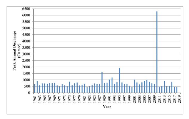
Fig. 2: Peak Annual Discharge Recorded at River Swat (Chakdara Station)
