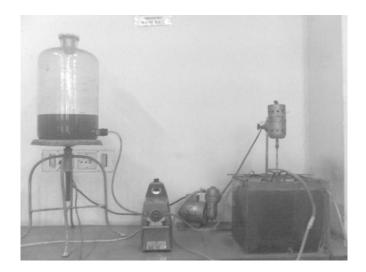
Fig 2b: Laboratory setup of biological reactor used in this study
