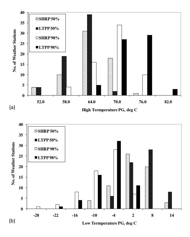
Figure 3 Histogram of High/Low Pavement Temperatures for 64 Stations
