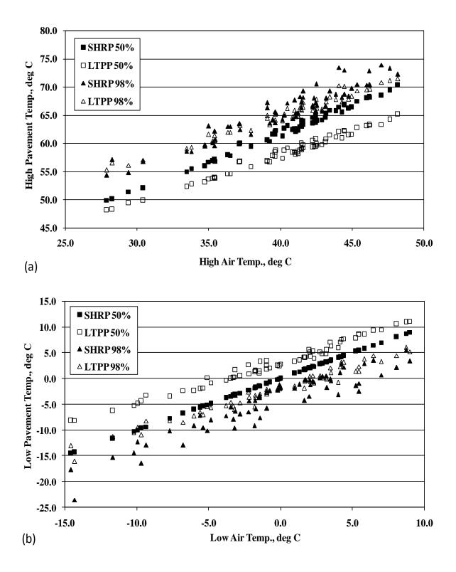
Figure 2 High and Low Pavement Temperatures as a Function of Air Temperature
