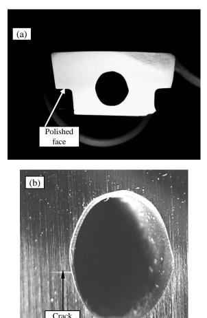
Figure 2: (a & b): Photograph showing the location and orientation of cracks in Blade # 1. The crack became visible to naked eye even before the final stage of polishing.
