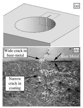
**Figure 3:** Scanning-Electron-Micrograph taken by tilting the specimen in such a manner that both the metallographically-polished surface as well as a part of the inside surface of the air-inlet hole could be seen. The scanned portion of the two surfaces which were essentially at right angle to each other are schematically illustrated in Figure 3a.
