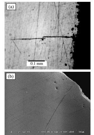
Figure 6: (a & b): Optical and Scanning Electron Micrographs taken from another location of Blade # 2, illustrating that the cracks are not exposed to surface, and hence cannot be related to corrosion fatigue. It may also be noted that in addition to the small crack just beneath the surface, there are two more independent sub-surface cracks.
