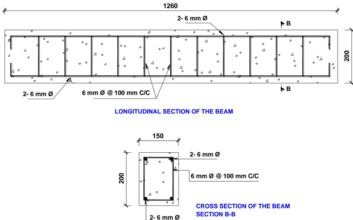
Figure 2: Reinforcement details of test specimen
