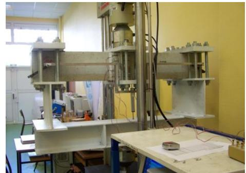
**Figure 3:** Experimental setup for reverse cyclic bending test on beam
