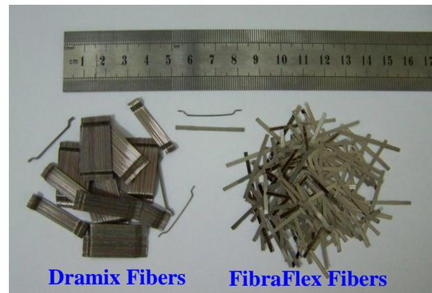
**Figure 1:** Metallic fibers used in this study
