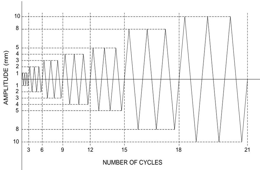
Figure 4: History of the displacement controlled reverse cyclic loading
