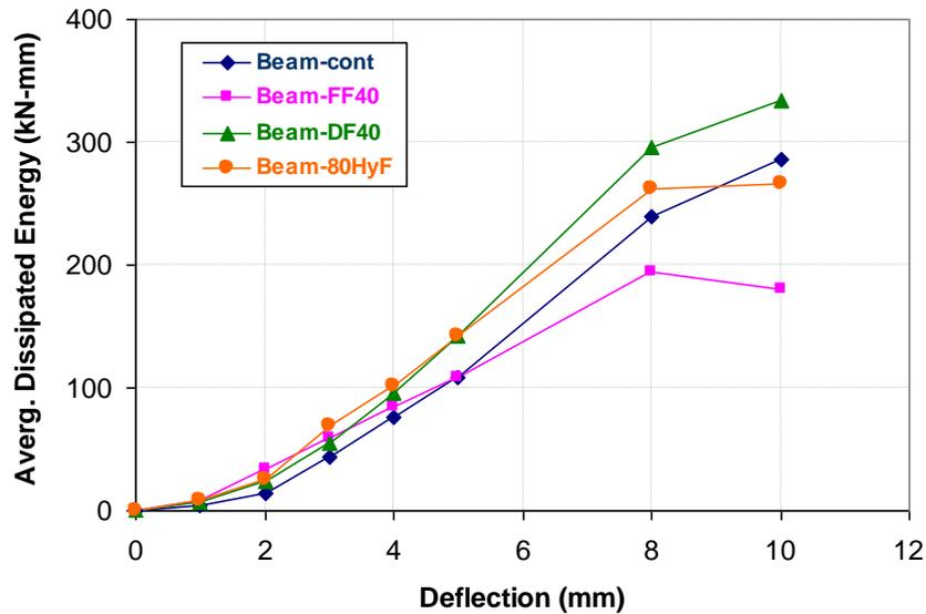
**Figure 9:** Average dissipated energy of all tested beams
