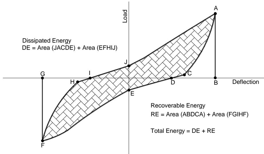
**Figure 8:** Typical loading cycle for a structural element
