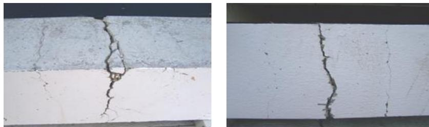
Figure 6b: Spalling of concrete cover (Fibrous Beam)
