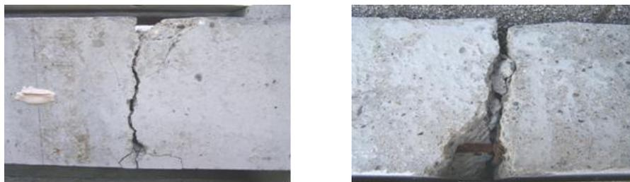
Figure 6a: Spalling of concrete cover (Control Beam)
