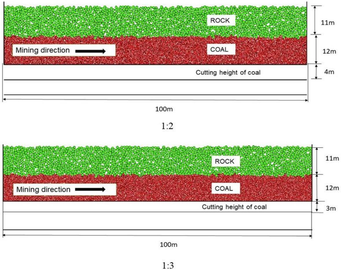
Fig. 6: PFC2D numerical models for effective caving process at 1:2 and 1:3
