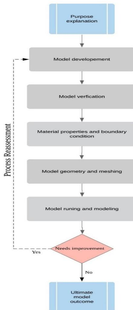
**Fig. 5:** Flow chart of general modeling procedure
