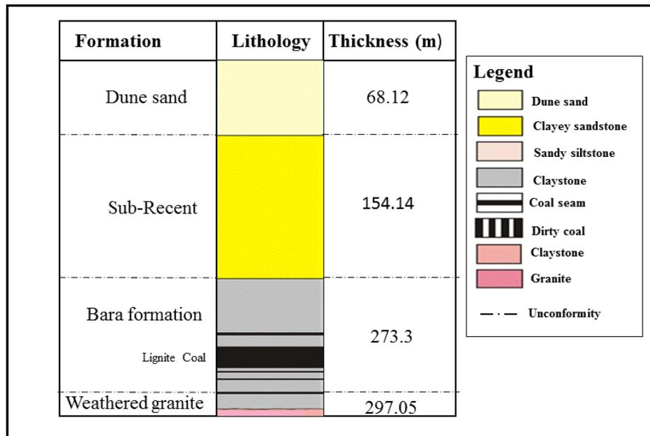
**Fig. 4:** Generalized stratigraphic column of Block-IX Thar Coalfield
