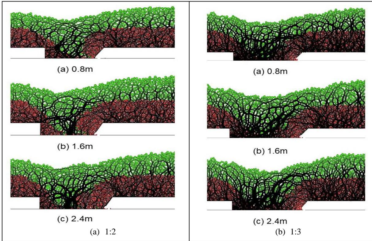
**Fig. 9:** The developing of chain force during the drawing process
