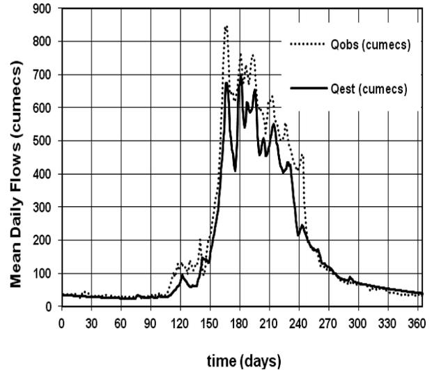
Fig.10: Validation of UBC Model for year 1996
