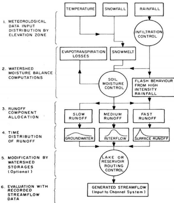
Fig. 2: UBC watershed model generalized flow chart
