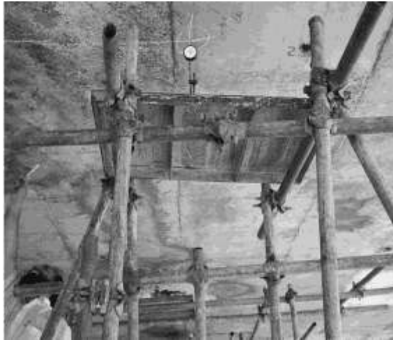
Fig. 3 Deflection Gauge Installed at the Center of Panel
