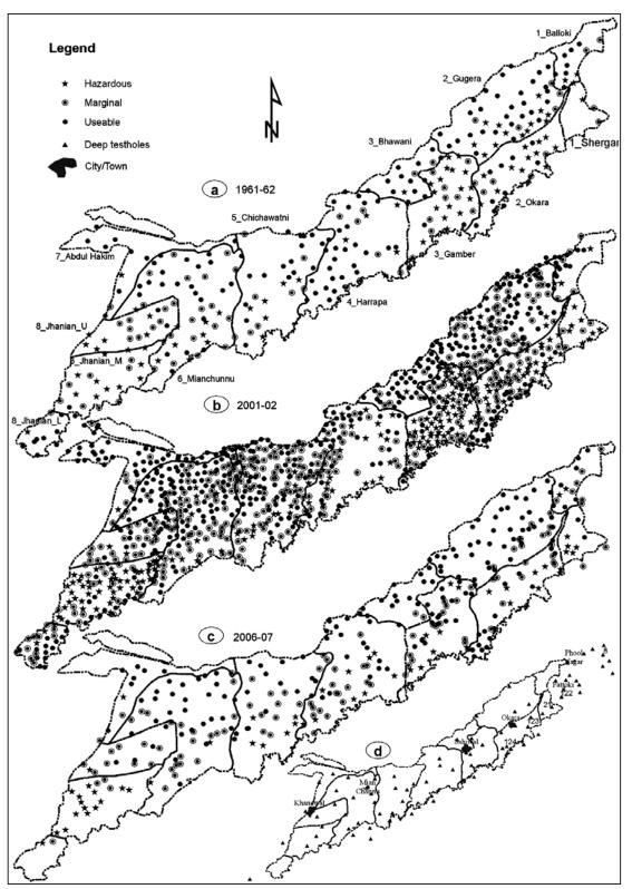
Fig. 4: Groundwater quality as observed on a:1961-62; b:2001-02; c:2006-07; & d:test hole locations (1961-62).
