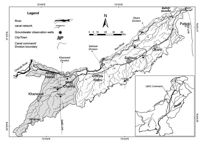
Fig. 1: LBDC canal irrigation network managed through four Irrigation Divisions.
