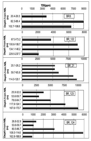
**Fig. 6:** Groundwater salinity profile for the strip from Raiwind to middle of Okara & Sahiwal (left side of Lahore-Multan road).
