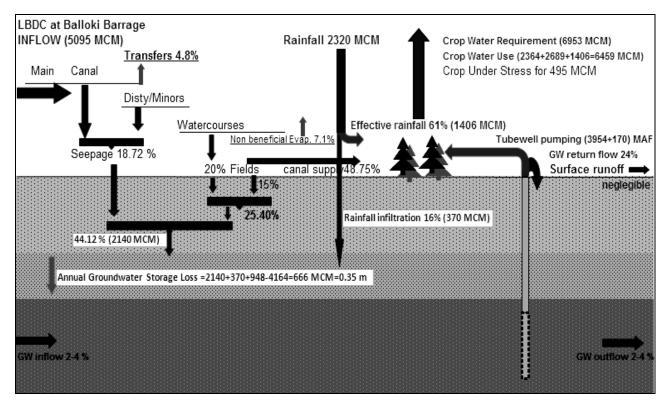
Fig.9: Crop water requirement, surface water and groundwater balance in LBDC command (irrigation system efficiencies adopted from [9].
