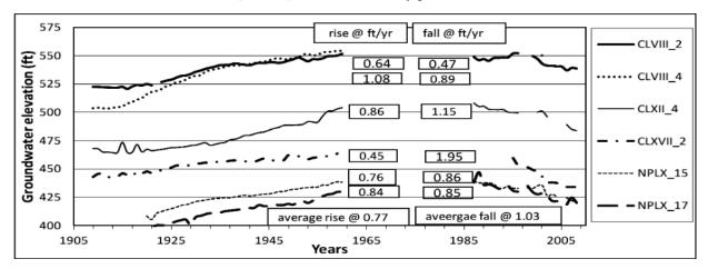
**Fig. 2:** Groundwater hydrographs spanned over one century, showing reservoir filling and depletion in LBDC command (1961 to 1986 is data gap).
