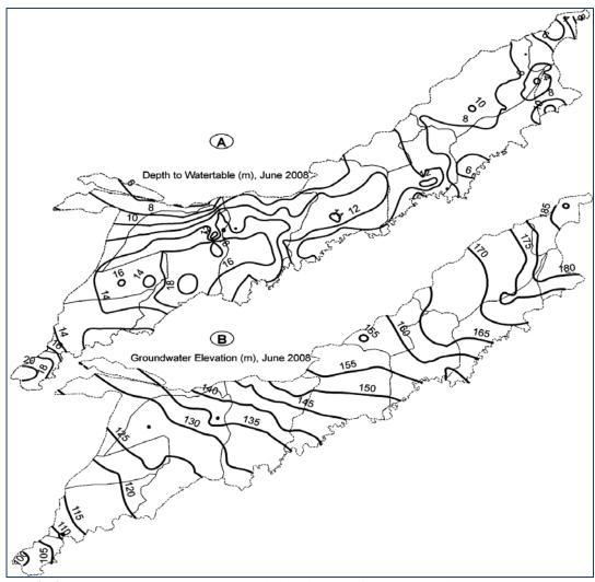
Fig.3: Depth to groundwater (A); and elevation (B), for June 2008 in LBDC command.
