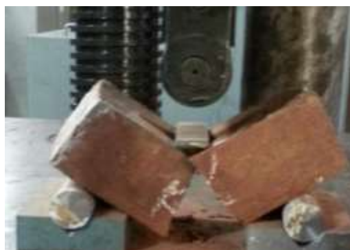
Figure 20: Failure of brick specimen during flexural testing
