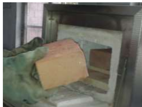
Figure 10: Brick specimens removed from electric oven after burning process
