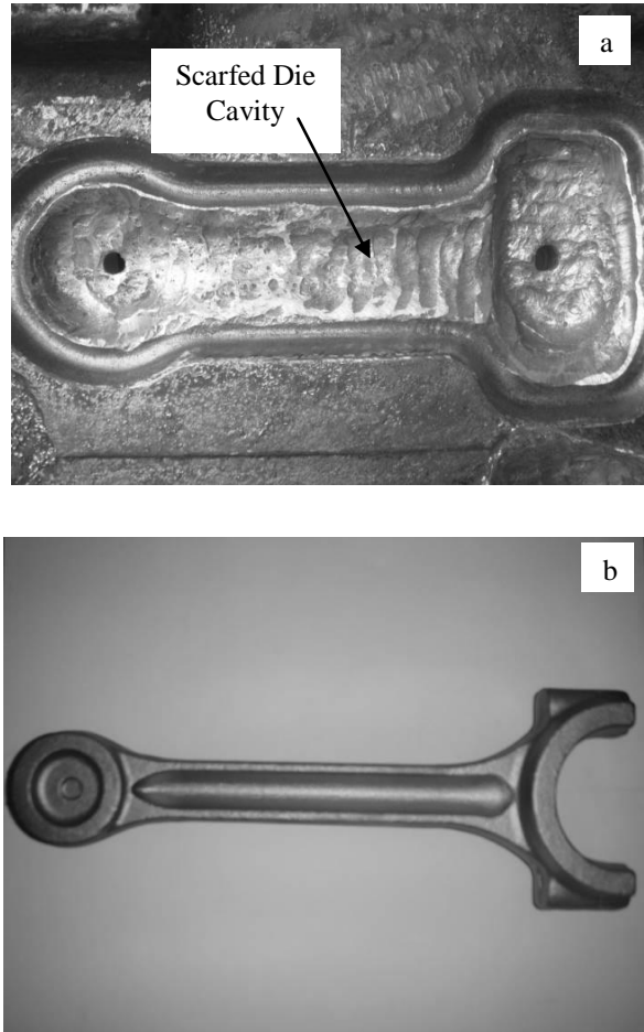
Fig.2 Photograph of Scarfed die of Connecting Rod (a), and forged Connecting Rod (b)
