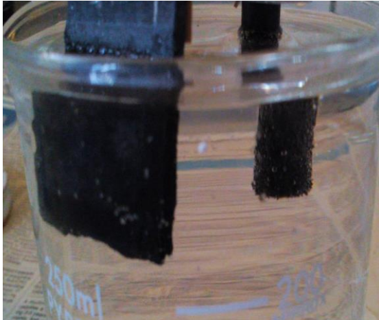
Figure 1: Nitric Acid + Tartaric Acid + Lead as Electrolyte
