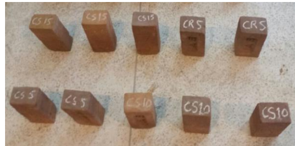
Figure 6: Brick specimens showing efflorescence results after 7 days.
