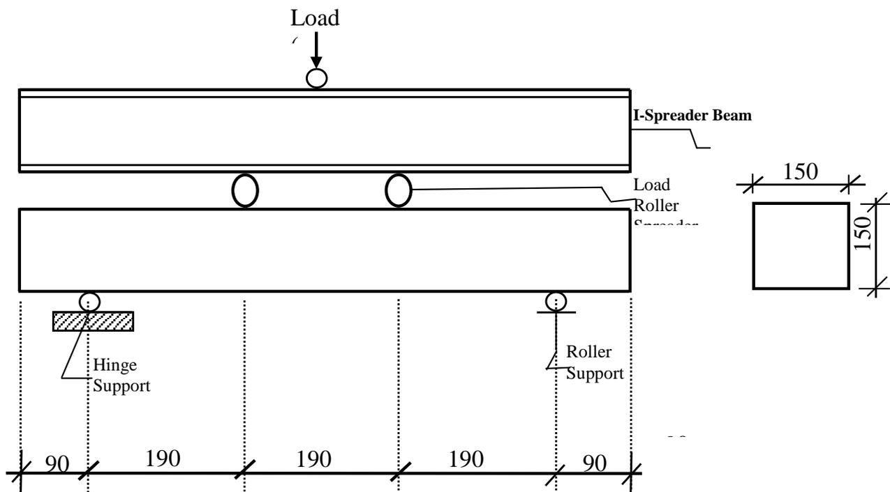
**Fig. 1:** Typical Beam and Loading Arrangement (Load is in KN, and dimensions in mm)
