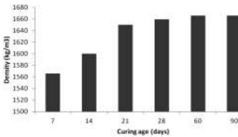
**Fig. 4** Variation of Dry Density with Curing Age for 5% cement replacement with pulverized bone
