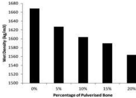
**Fig. 2** Effect of pulverized bone on density of foamed concrete
