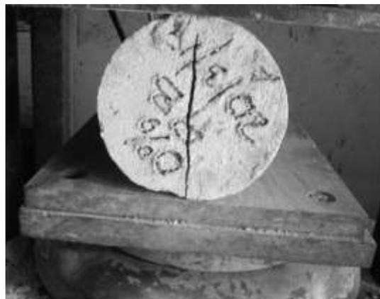
**Fig. 10** Cracking of the Cylinder Specimen
