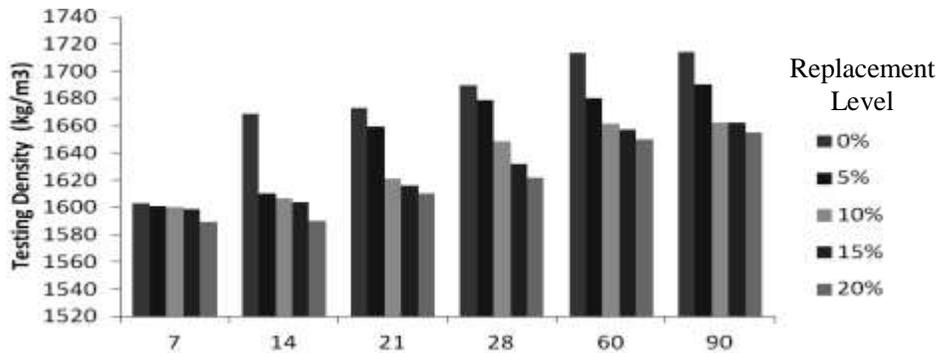
**Fig.3a** Curing Age (Days) for Water-Cured Specimens
