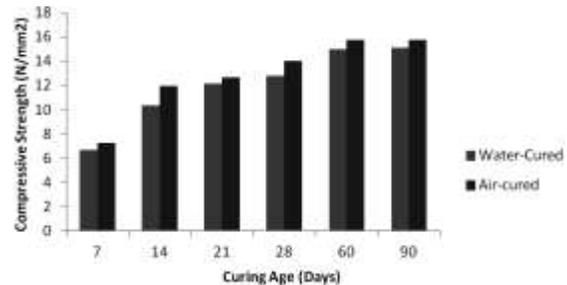
**Fig. 6** Effects of Curing Method of Strength Development (10% pulverized Bone Content)
