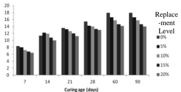
Fig.7b Effect of Curing Age on Strength Development (Ai-Cured Specimens)
