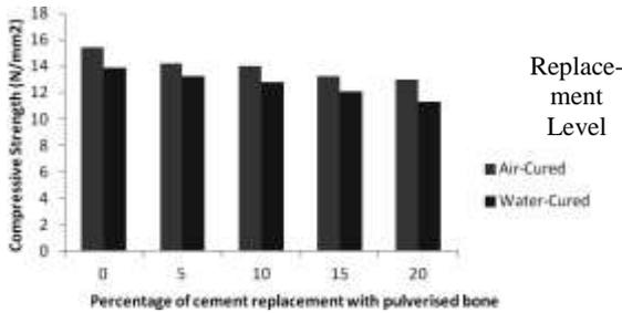
**Fig.8** Variation of Compressive Strength with Pulverized Bone
