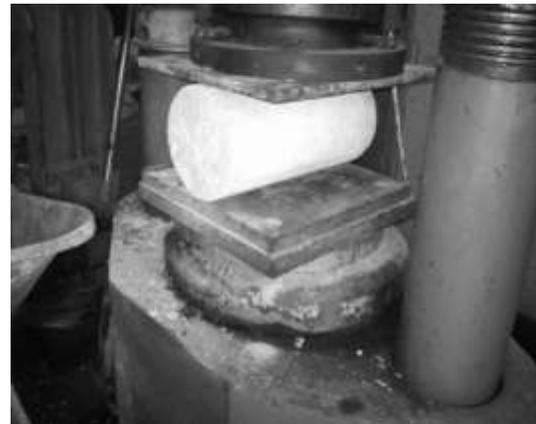
**Fig. 9** Splitting Test Arrangement
