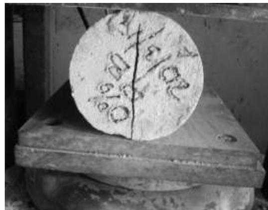
**Fig. 10** Cracking of the Cylinder Specimen
