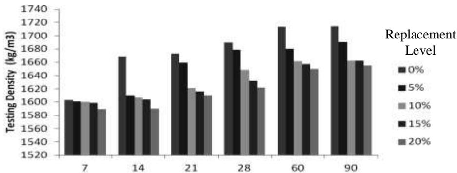
**Fig.3a** Curing Age (Days) for Water-Cured Specimens
