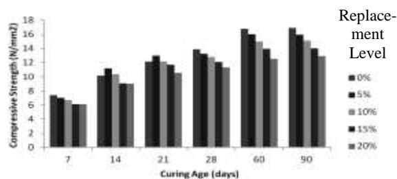
Fig.7a Effect of Curing Age on Strength Development (Water-Cured Specimens)
