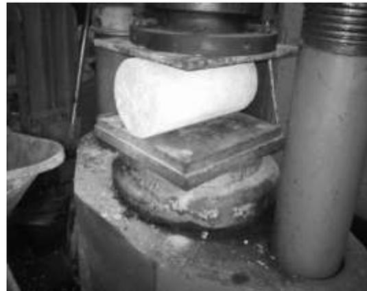
**Fig. 9** Splitting Test Arrangement
