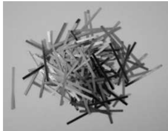
Fig.1: Amorphous metal fibers (FibraFlex)
