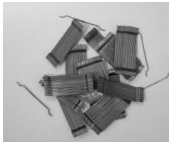
Fig.2: Carbon steel hooked-ends fibers (Dramix)
