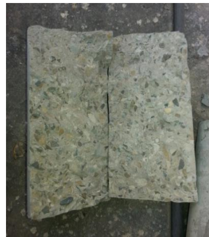
Fig. 11 Splitting of specimen into two pieces during tensile test
