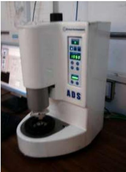
**Figure 2:** Bohlin dynamic shear rheometer (Asphalt and Concrete Mix Design Lab, Department of Transportation Engineering and Management, U.E.T. Lahore)
