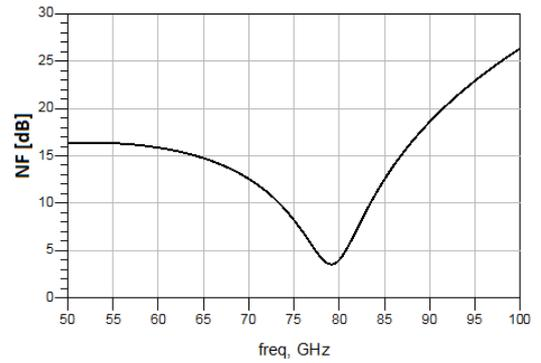
Fig. 7: Noise Figure for three stacked LNA.
