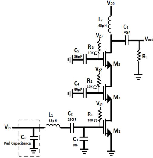
Fig. 3: Schematic of three stacked LNA
