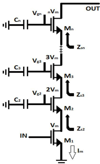
Fig. 1: n-Stacked FET configuration
