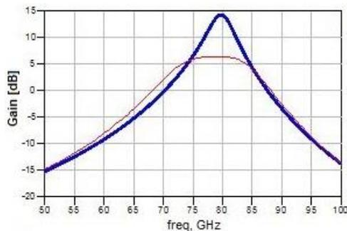
**Fig. 27:** Gain Vs Frequency graph after compensation
