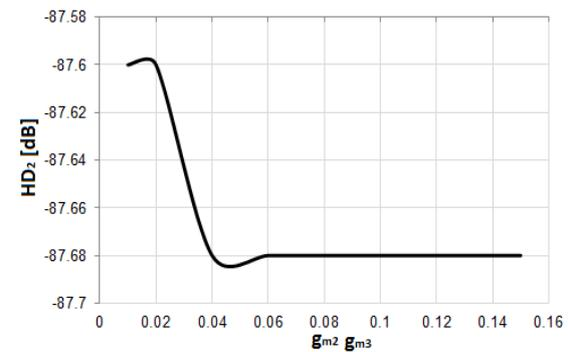
**Fig. 15:**  $g_{m2}$  and  $g_{m3}$  vs. HD2 Curve
