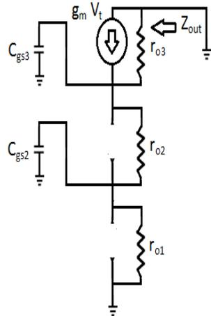
**Fig. 22:** Small signal equivalent circuit used for Blackman analysis
