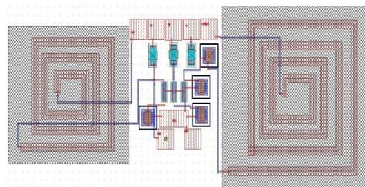
**Fig. 28:** Layout of the Purposed Three stacked LNA
