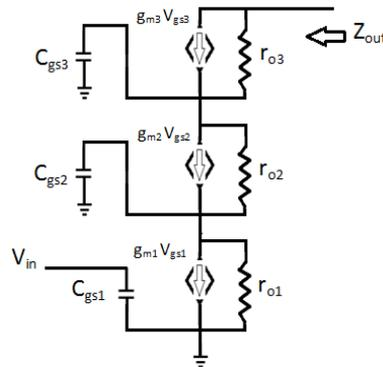
**Fig. 20:** Small Circuit equivalent of three stage stacked amplifier
