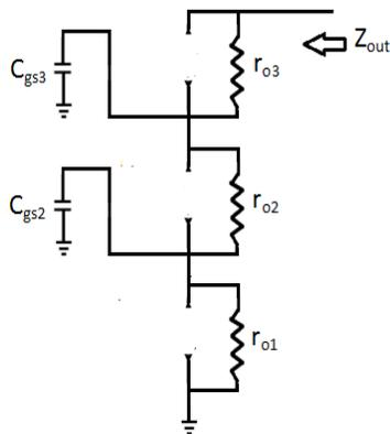
**Fig. 21:** Small circuit equivalent circuit of three stage stacked amplifier with  $g_m=0$
