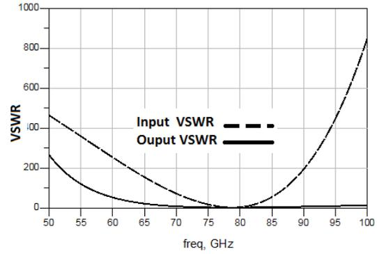
Fig. 6: VSWR for the 77-79 GHz three stacked LNA.
