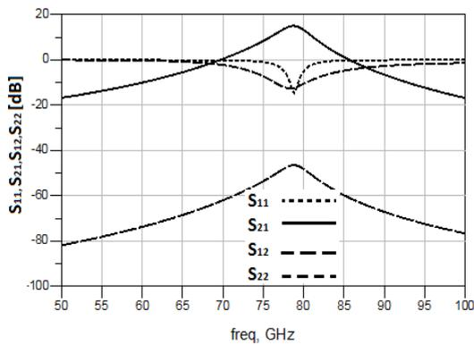
Fig. 5: S-parameters for the 77-79 GHz three stacked LNA.
