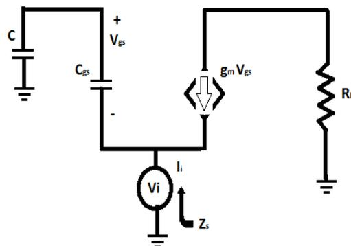
Fig. 2: External gate capacitance effect on FET's source impedance.
