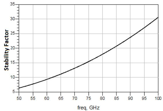
Fig. 8: Stability Factor of three stacked LNA.
