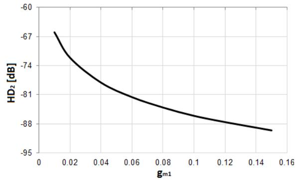
**Fig. 14:**  $g_{m1}$  vs. HD2 Curve
