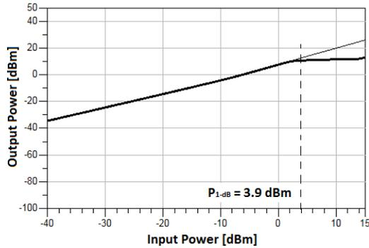
Fig. 9: 1-dB compression point curve
